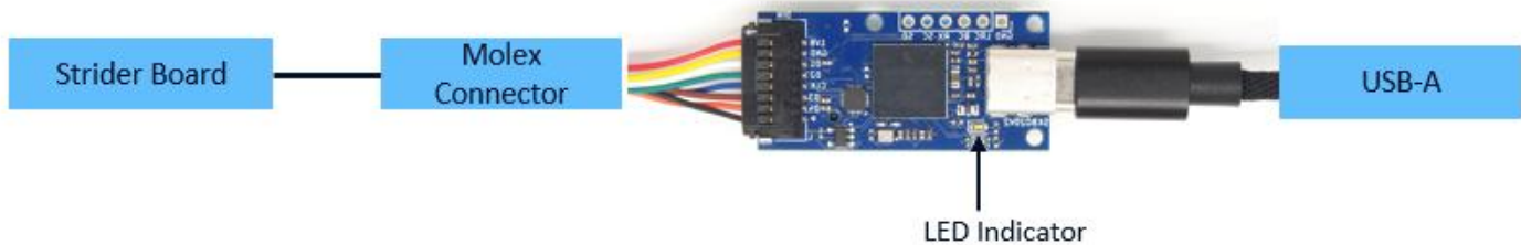
Figure 3: PARDI Audio Interface Board
