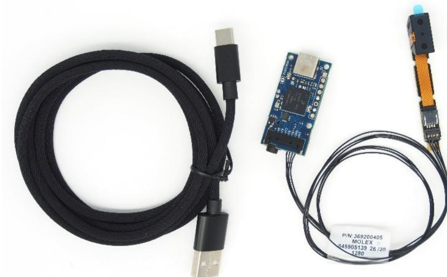
Figure 1: Soundskrit Module Demo Kit (Scarab-1600)
