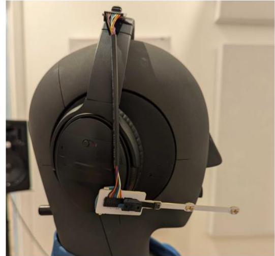
Figure 6: Mantis board with cable routed over the headband
