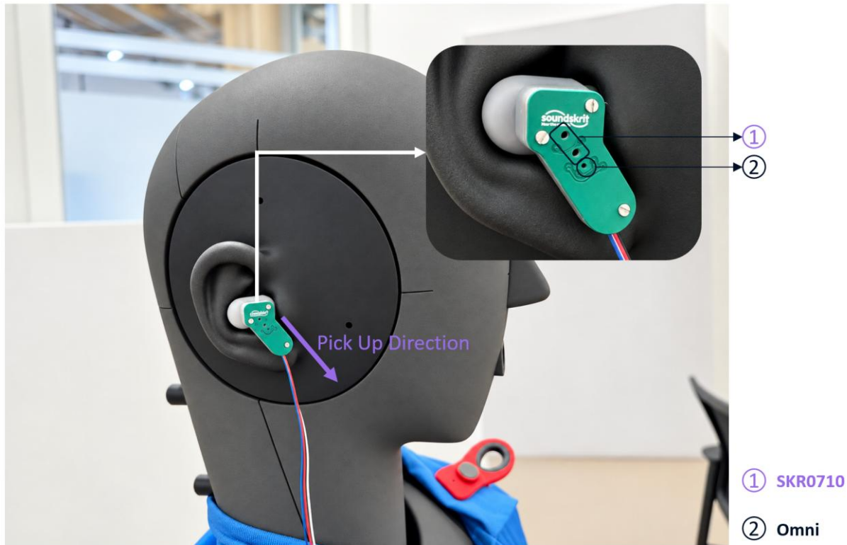
Figure 2: Cicada Microphone Locations and Directions
