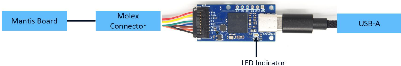
Figure 3: Mantis PARDI Board Interface
