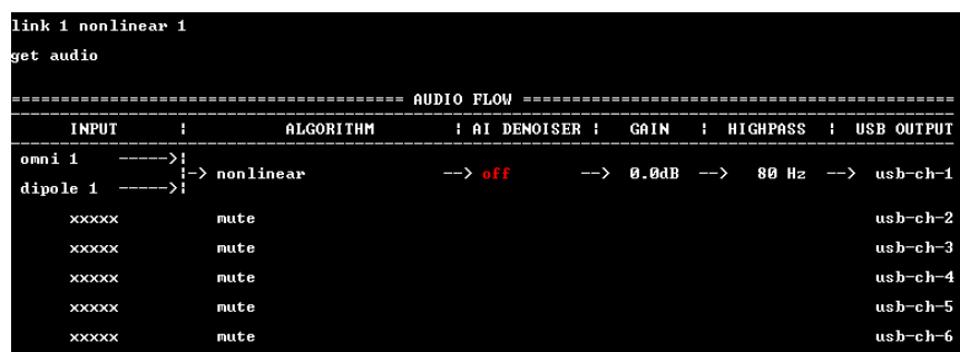
Figure 20: Example: routing the long boom nonlinear beam to USB channel 1.
