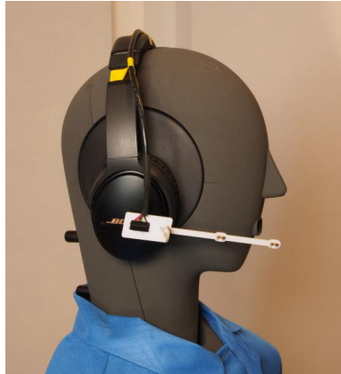
Figure 15: Mantis board positioned near the corner of the mouth
