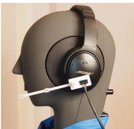
Figure 2: Boom microphone prototype featuring a pair of microphones (dipole + omnidirectional).
