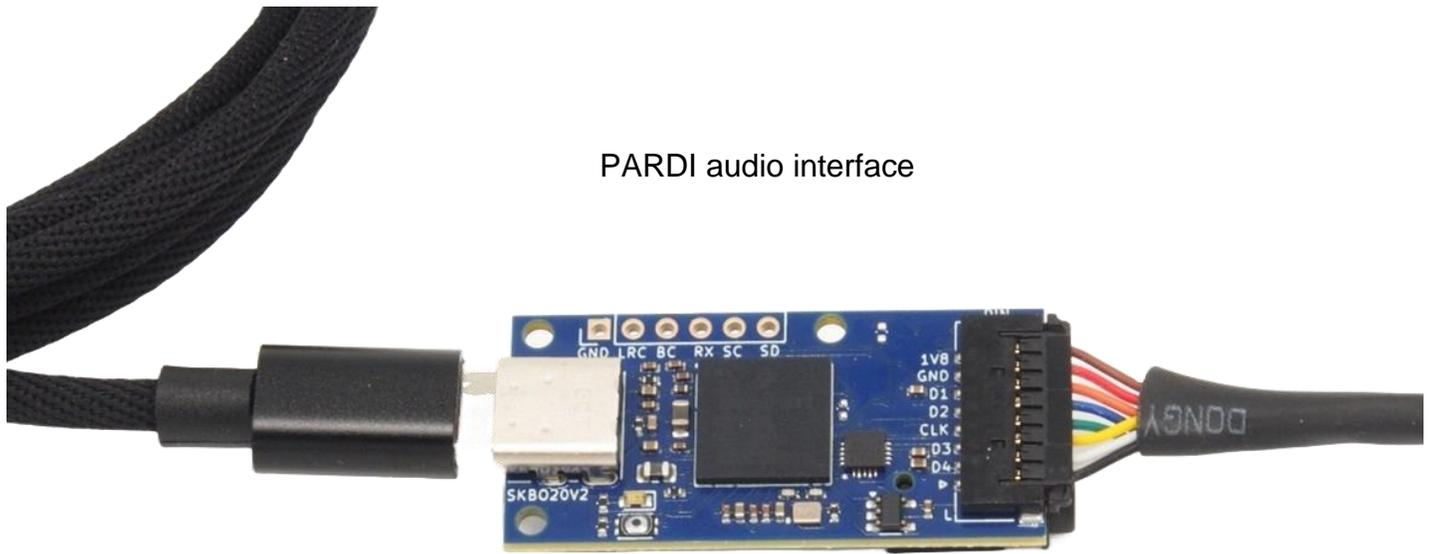
Figure 7: Connection of the Soundskrit multichannel audio interface.
