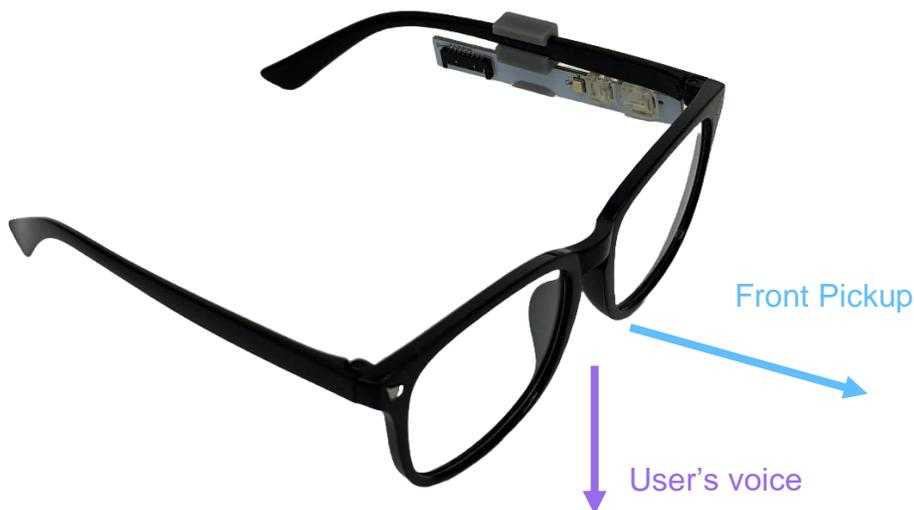
Figure 6: Cricket glasses with microphone PCBs on each side. Only the left side is used. The arrows illustrate the directional beams processed by the GUI for capturing the user's voice (towards the mouth) and front speech (forwards).
