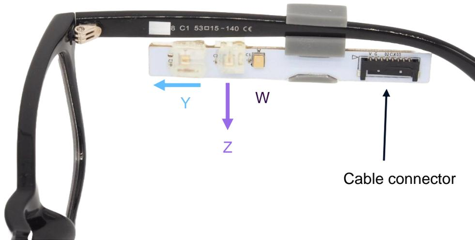
Figure 5: The PCB holds a forward-facing dipole (Y), a downward-facing dipole (Z), and an omnidirectional microphone (W). The connector for the cable to the PARDI audio interface is located at the back. (Note: Although PCBs may be present on both sides, only the left side is active for this demo).
