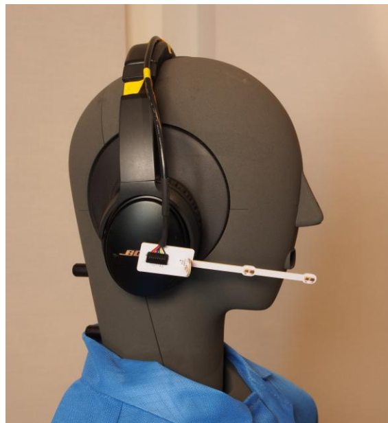
Figure 9: Mantis board with cable routed over the headband
