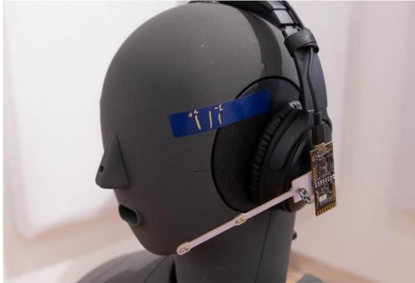
*Figure 13: Mantis board positioned near the corner of the mouth*
