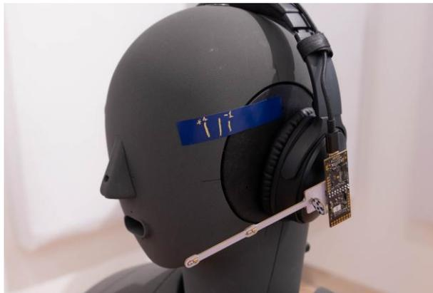
Figure 8: Mantis board with cable routed over the headband
