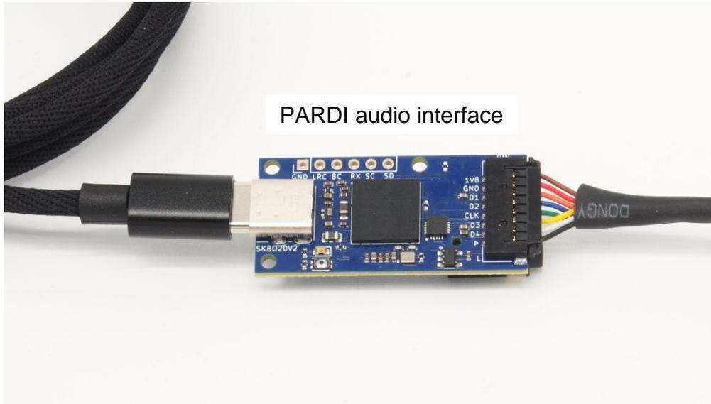
*Figure 15: Connection of the Soundskrit multichannel audio interface.*
