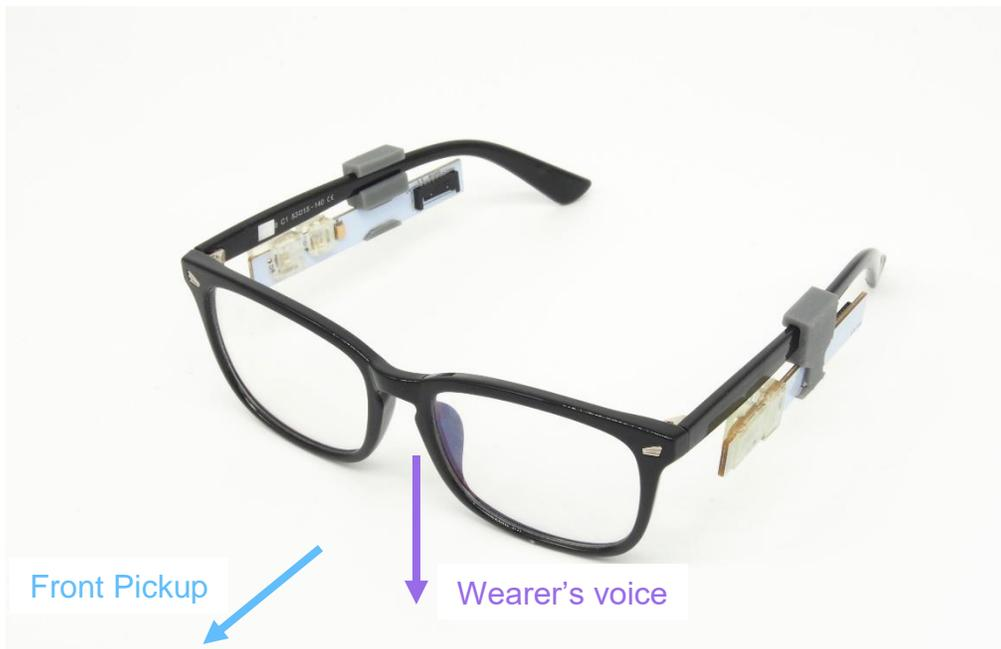
Figure 14: Cricket glasses with microphone modules on each side. Only the left module is used currently in the GUI. The arrows show the beam directions outputted from the GUI: The wearer's voice and front speech pickup.
