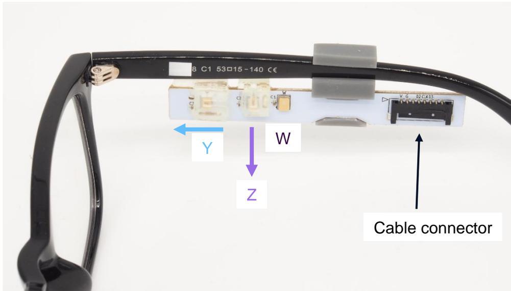
Figure 13: Each microphone module holds a forward-facing dipole microphone (Y), a downward-facing dipole microphone (Z) and an omnidirectional microphone (W). At the back of the module is a connector for the cable to the audio interface.
