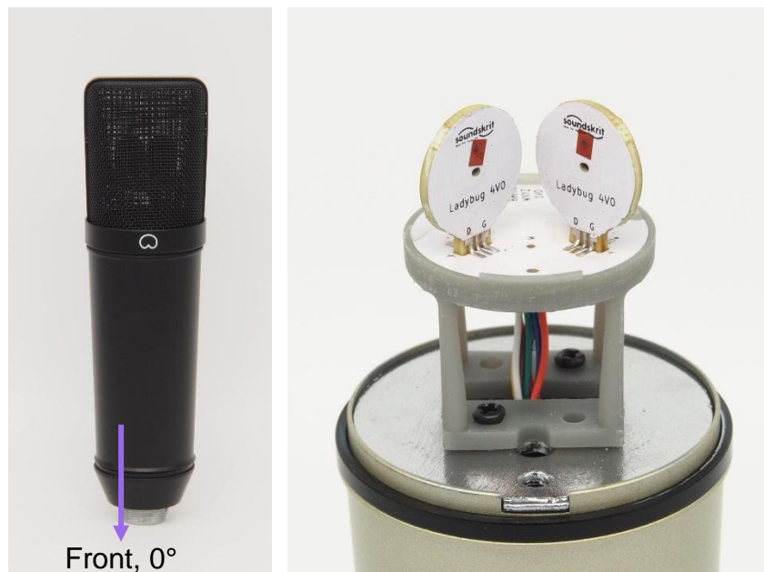
Figure 3: Microphone shell with Soundskrit Beetle integrated (left). Beetle PCB without microphone screen (right).
