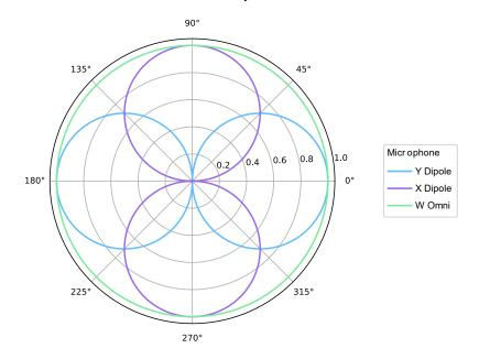
This array allows for features described in the "Introduction to the XY configuration using MEMS directional microphones" article and the beamforming ability described in the "How do microphones combine to create new polar patterns?" article. In addition to DOA, a WXY array includes stereo audio pickup, 360° beam steering and beamforming features.
