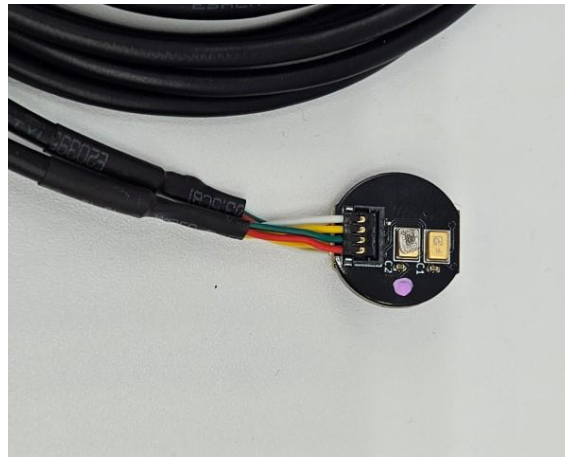
Figure 1: Dipole + omnidirectional microphone PCB
