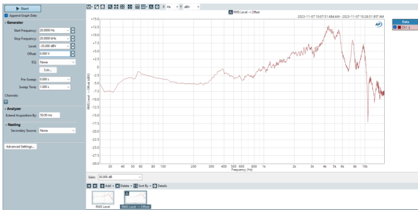
Figure 12: Frequency Response of Measured DUT (SKR0400)
