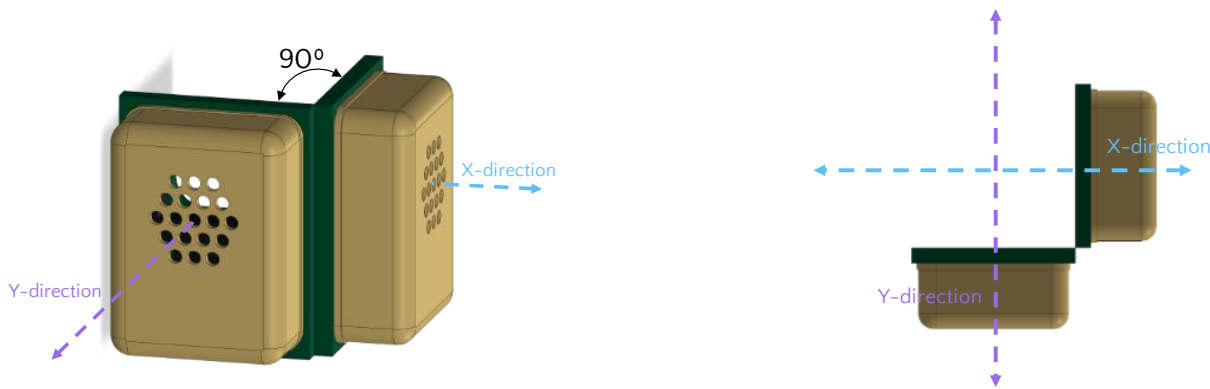
Figure 8: Two Soundskrit microphones for 360° sound capture in perspective view (left) and top view (right)
