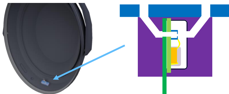
Figure 3: Example of microphones inside of a headset earcup
