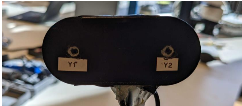
Figure 5: Webcam with 2 front-face Soundskrit Microphones
