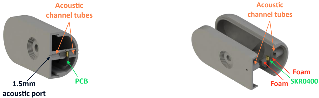
Figure 3: Cross section (left) and exploded view (right) of Soundskrit Microphones in a Webcam
